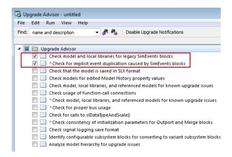
The graphic shows the SimEvents checks in Upgrade Advisor. In the previous release, these checks were directly listed under **Upgrading to the Current Simulink Version** in the Model Advisor.
