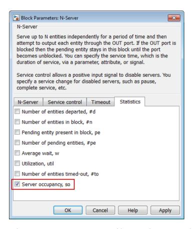
Selecting **Server occupancy**, **so** adds a signal output port labeled **so** to the block.
