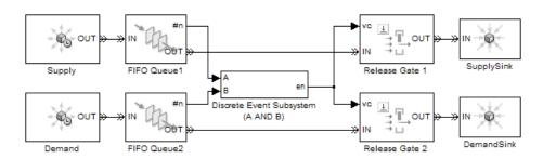
Suppose that the top queue contains one entity and an entity arrives at the previously empty bottom queue. Assuming that no block in the model has its **Resolve simultaneous signal updates according to event priority** parameter selected, the entity arrival has the following cascade of consequences:
